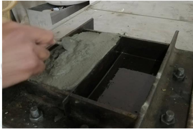
The Mold used to cast samples for thermal conductivity test
