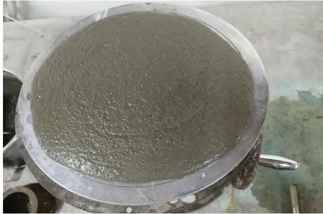
Followability of mortar used to prepare foam concrete According to ASTM C 230
