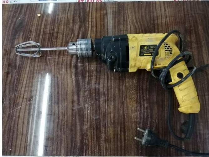
the Drill used to performed the foam
